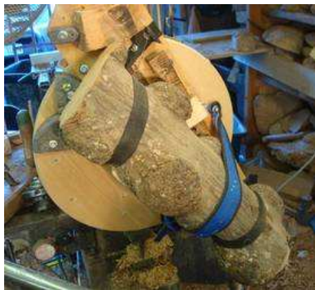
Fig 2. Showing counterweight and sled mounted on backing plate
